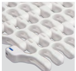
S.201 Open radius belt with a very low collapse factor. Can run in S- and J-curves for spiral coolers/freezers as well as normal radius applications.
