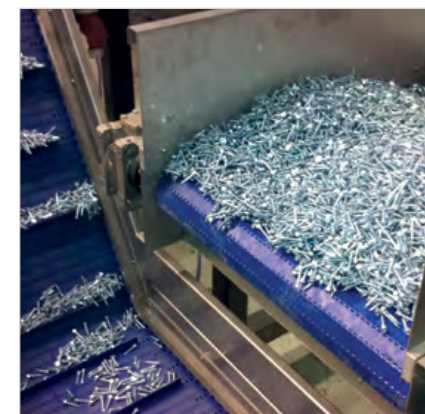
25-402 Raised ribs for minimum product contact. Air circulation under product. Easy to clean
