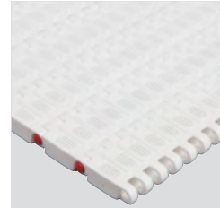
25-413 Perforated surface with 1 x 6 mm openings. 1.2 mm longitudinal flights to "lift" products.
