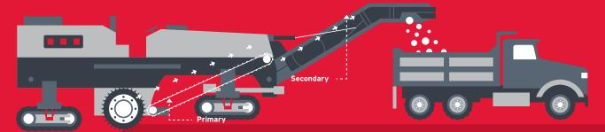
Road milling machines remove asphalt from roads in order to repair damaged sections of streets and highways. The asphalt is removed by a large cutting drum, then fed onto the primary/pickup belt. This belt feeds the material from the primary belt to the secondary/discharge belt. The secondary belt then feeds the reclaimed material into a dump truck.
