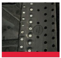
Super-Screw® fasteners combine the strength and dependability of a vulcanized splice without the costly downtime to fabricate an endless belt. With the ability to be installed on any conveyor belt, even in challenging access situations, this fastener is quick and easy to install.
