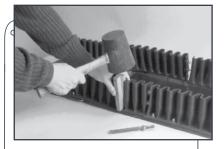
The two cemented surfaces must be stitched into close contact. Using a rubber mallet, pressure is best applied downward on a wooden block or blunt metal rod (not furnished). A firm surface under the belt in the area being stitched is required for best results.
