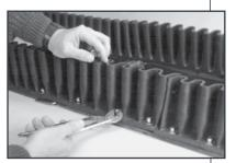
Completing the splice in the sidewall is accomplished by inserting the flat head bolts through each end of the rubber corrugations. Place fender washers and lock nuts in place and tighten appropriately.
